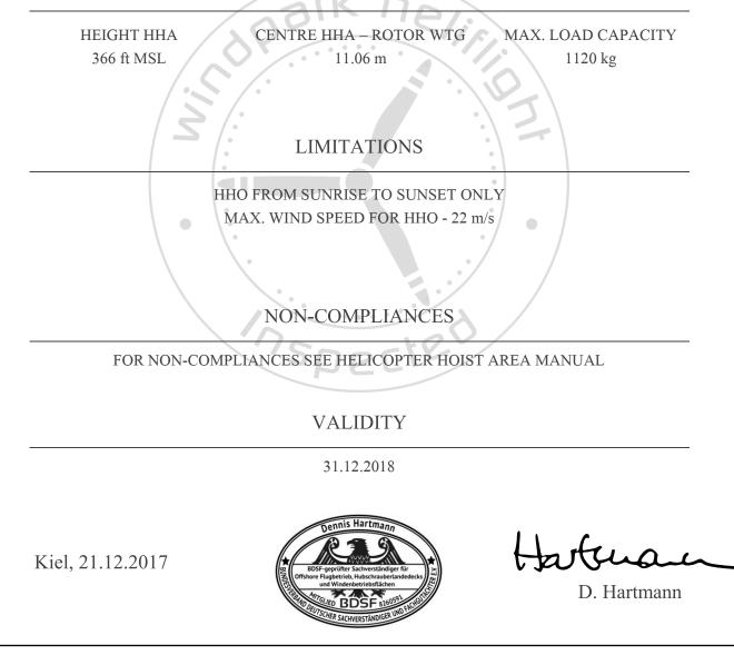
The operator of the hoist areas is fully responsible to ensure that the hoist areas and the related equipment are fit for purpose according to Gemeinsame Grundsätze. This certificate will cease to be valid if changes to a hoist area or the related equipment are being made without prior agreement with windpark heliflight consulting GmbH.
